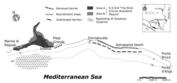
Fig. 6: Project of the recovery interventions on the littoral.
