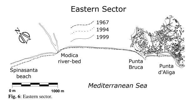
The beach is seen to have increased in the central sector as a result of the breakwater barriers, a comparison between the coastlines in the two periods considered (1967-1994; 1994-1999) reveals for the adjacent stretch of coast (Spinasanta beach) an incipient reduction in the beach area equal to about  $73.6 \cdot 10^3 \text{ m}^2$ . In the part stretching from immediately beyond Spinasanta beach as far as Punta Bruca, there was a
